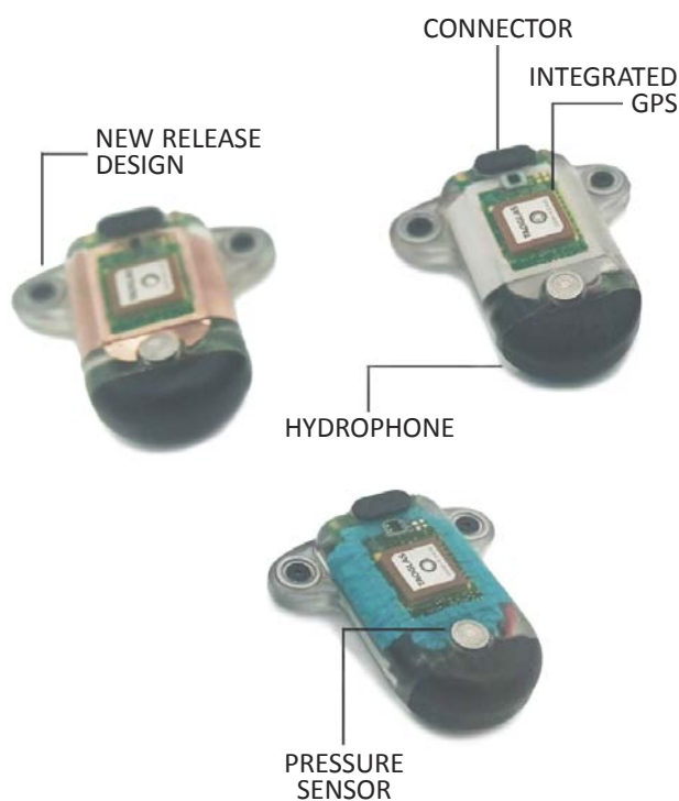
Figure 2: Images of the redesigned 2025 DTAG4 core units fabricated to support researchers conducting behavioral response studies using the LMR-supported mixed-DTAG. The redesign included improved features that were present in the 2025 version of the lease pool tags.
